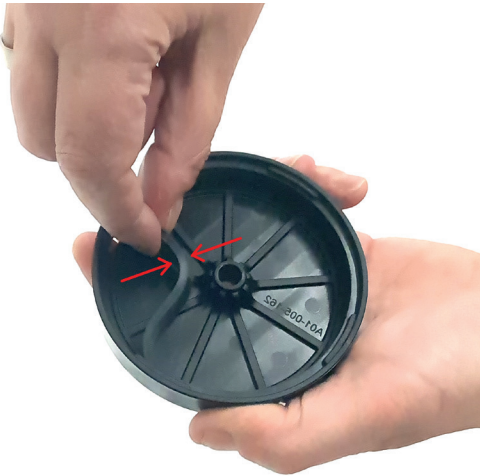
Picture: Removing the brake pad
