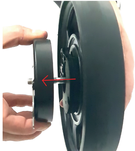
Picture: Removing the brake drum
